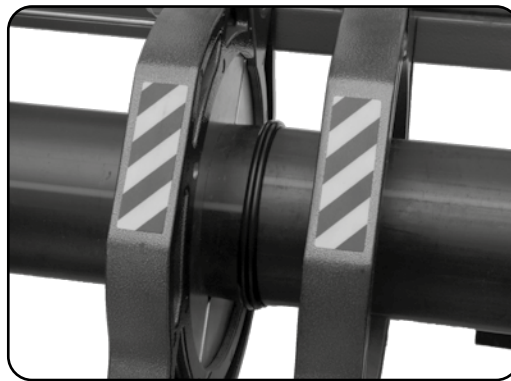
Figure 5: Pipe alignment and joining, beads appear under pressure
